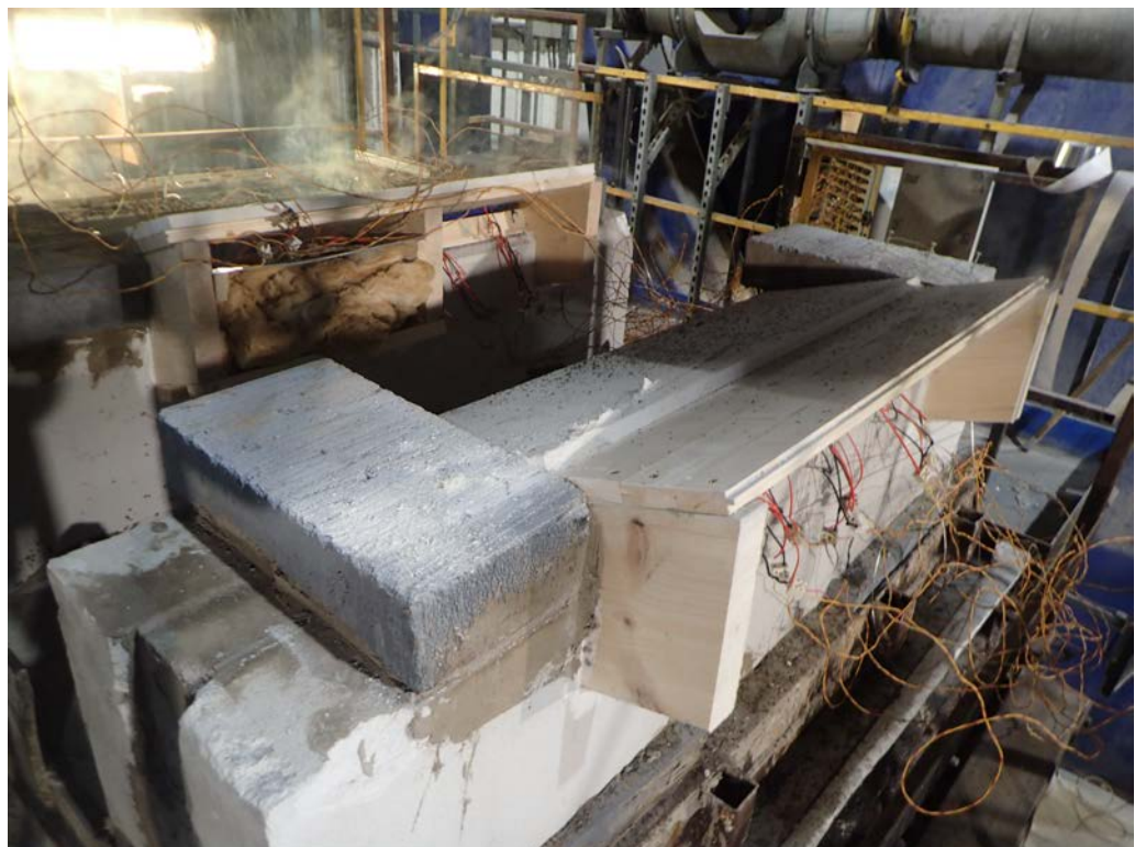
The unexposed face of the floor construction after a test duration of 15 minutes
